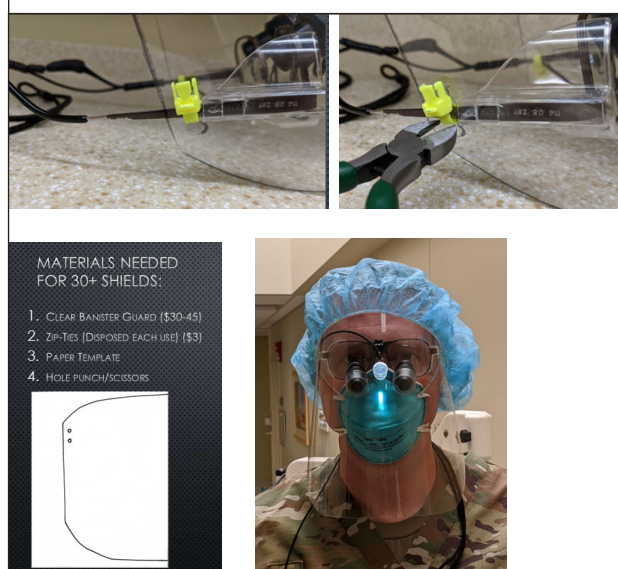
Figure 4. Fabrication of the locally constructed face shield.
